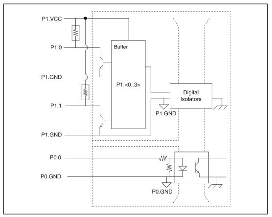
Figure 6-2. NI 6233 Digital I/O Connections (DO Sink)
